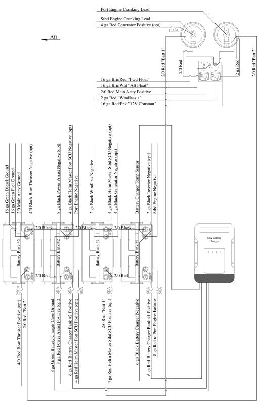
NOTE 1: Engine isolator fuse changes to 100A MRCB if the boat is equipped with V6 engines.
